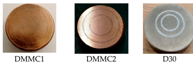
Figure 9. Wear scars on disks after test.
