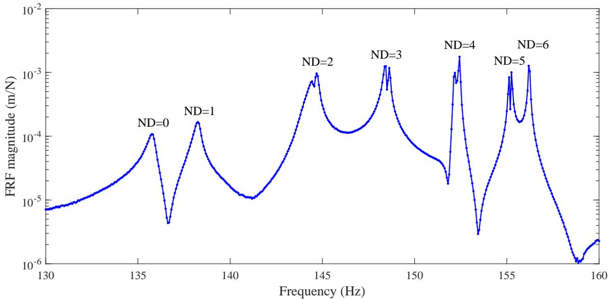
Figure 17: FRF obtained by hammer test for blade 1.
