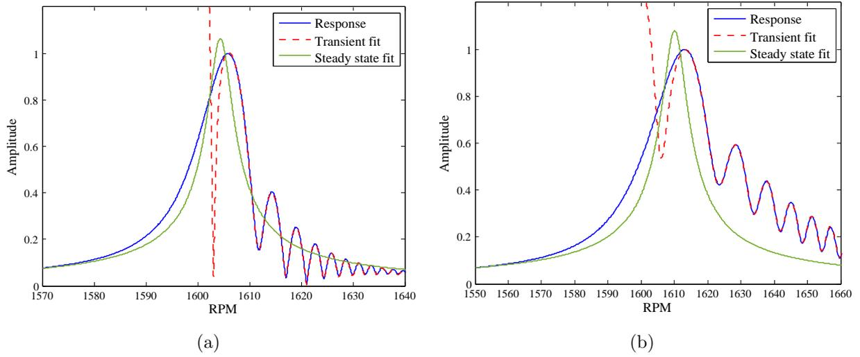
Figure 10: Amplitude obtained by the steady state and transient models for two rotating speed sweep rates and  $\zeta = 0.001$  at EO=6, ND=6 and, (a) 0.125 Hz/s, (b) 0.50 Hz/s.
