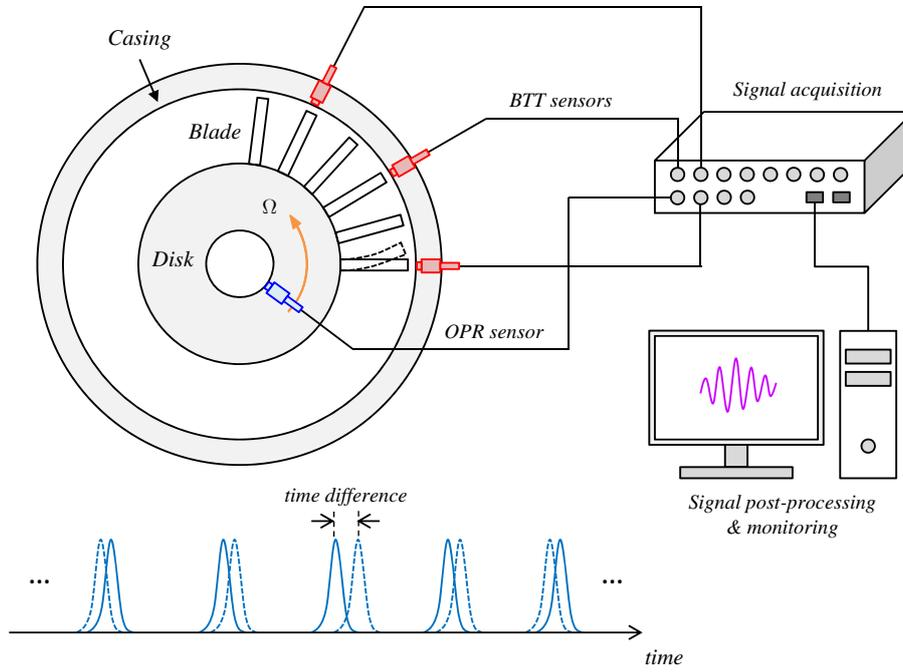
Figure 2: Schematic illustration of a BTT measurement system.
