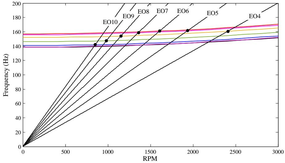
Figure 16: Campbell diagram of the test case.
