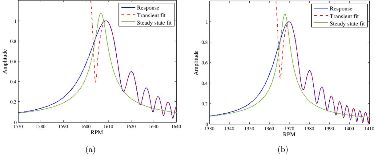
Figure 9: Amplitude obtained by the steady state and transient models for two different resonance cases at the rotating speed sweep rate of  $0.25Hz/s$  and  $\zeta = 0.001$ , (a)  $EO=6$  ,  $ND=6$  , (b)  $EO=7$  ,  $ND=5$ .
