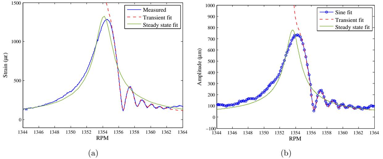
Figure 23: Fitting results for blade 1 corresponding to EO=7 and ND=5, (a) strain gauge, (b) BTT.
