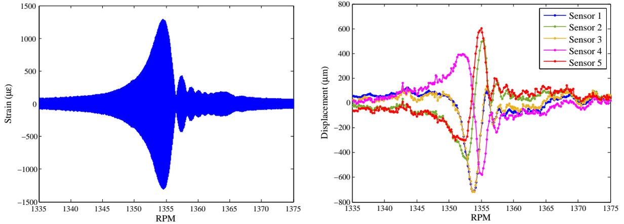
Figure 22: Strain and BTT displacement measurements for blade 1 corresponding to EO=7 and ND=5.
