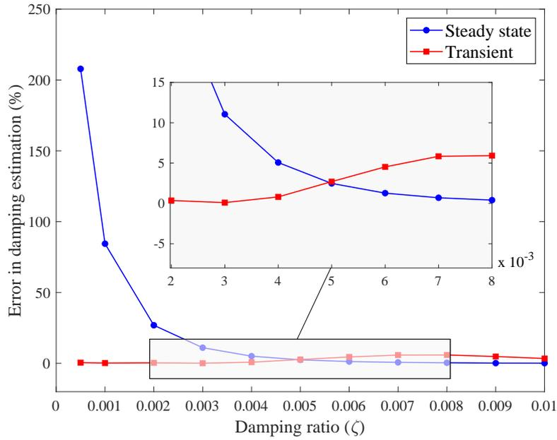
Figure 12: Errors in the damping estimation by the steady state and transient models for the rotating speed sweep rate of  $0.25Hz/s$  at  $EO=6$ ,  $ND=6$ .
