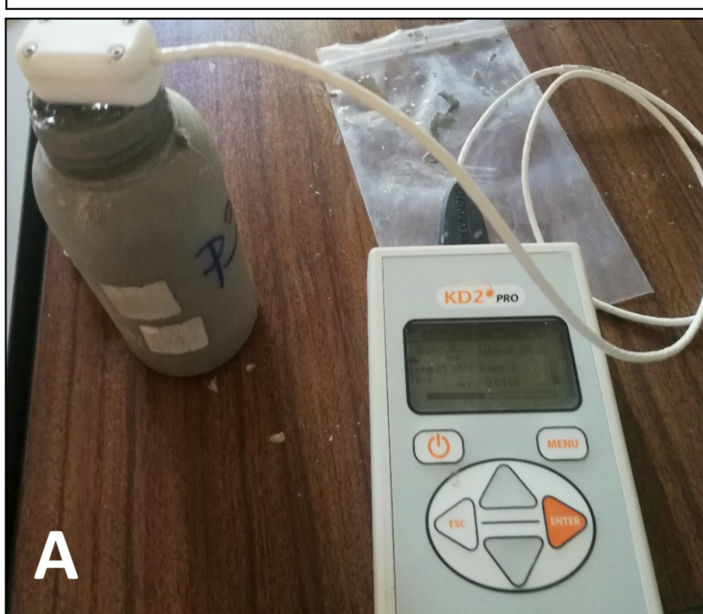
Fig. 2 A Temperature and thermal conductivity device; B: submersible temperature recorder
