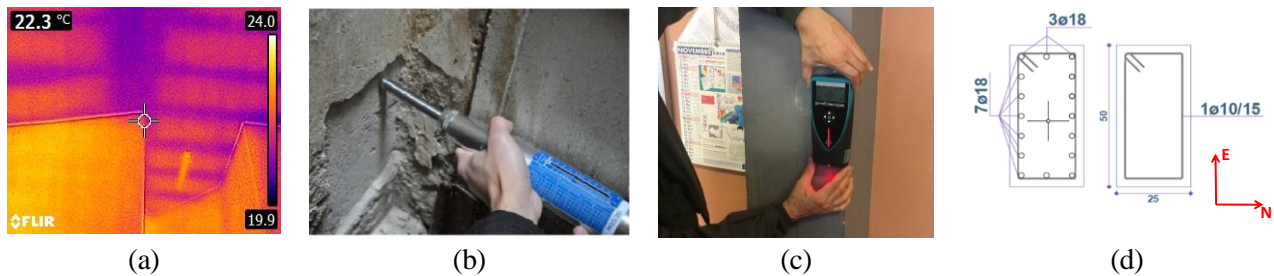
Figure 3. Thermal camera test (a), sclerometer test (b), pachometer test (c), and column cross section (d)
