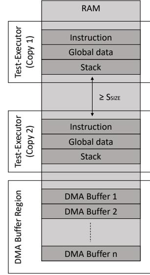
Fig. 5. Memory layout of the proposed software architecture.
