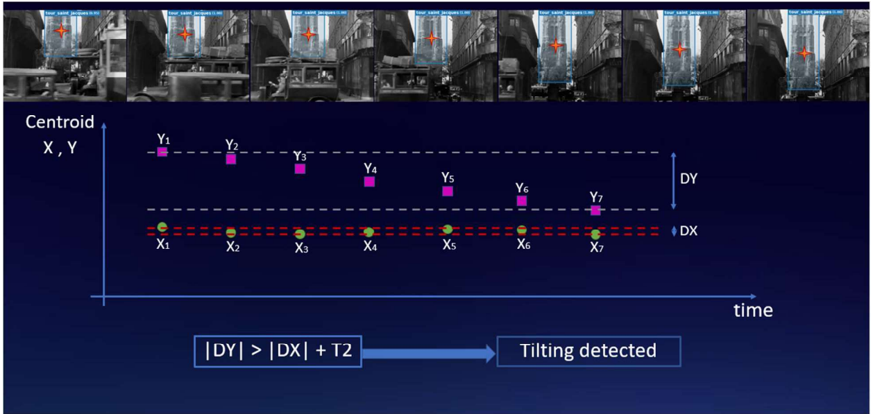
Figure 70. Results of the camera motion estimation step that recognised the “camera tilting” movement.
