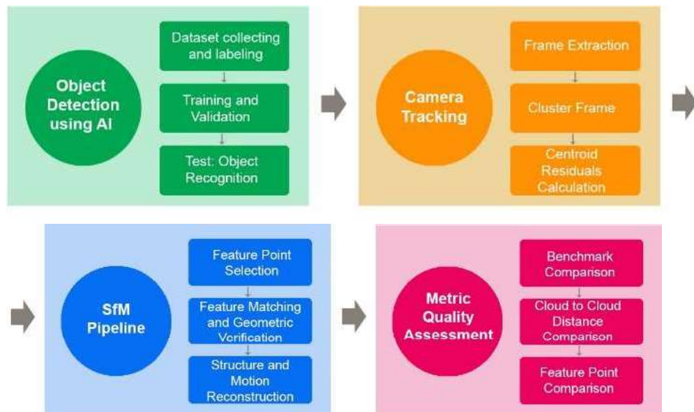
Figure 2. The proposed workflow: the first step is the object detection using AI, the second step (used only in case of video) is the camera tracking, the third step is the 3D reconstruction following the SfM pipeline and the fourth step is the metric quality assessment.
