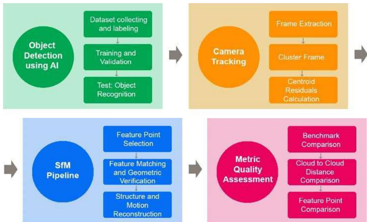
Figure 1. The general workflow proposed in this dissertation. The following sections will deal with the application of this workflow on historical film footage, focusing on the two steps of “object detection using AI” and “camera tracking”.
