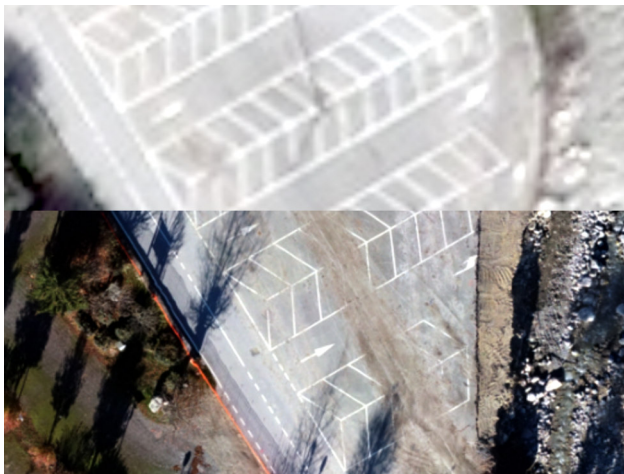
Figure 10. Qualitative evaluation of satellite orthoimagery (top) level of detail and 2D position accuracy with respect to UAS orthoimagery (bottom).
