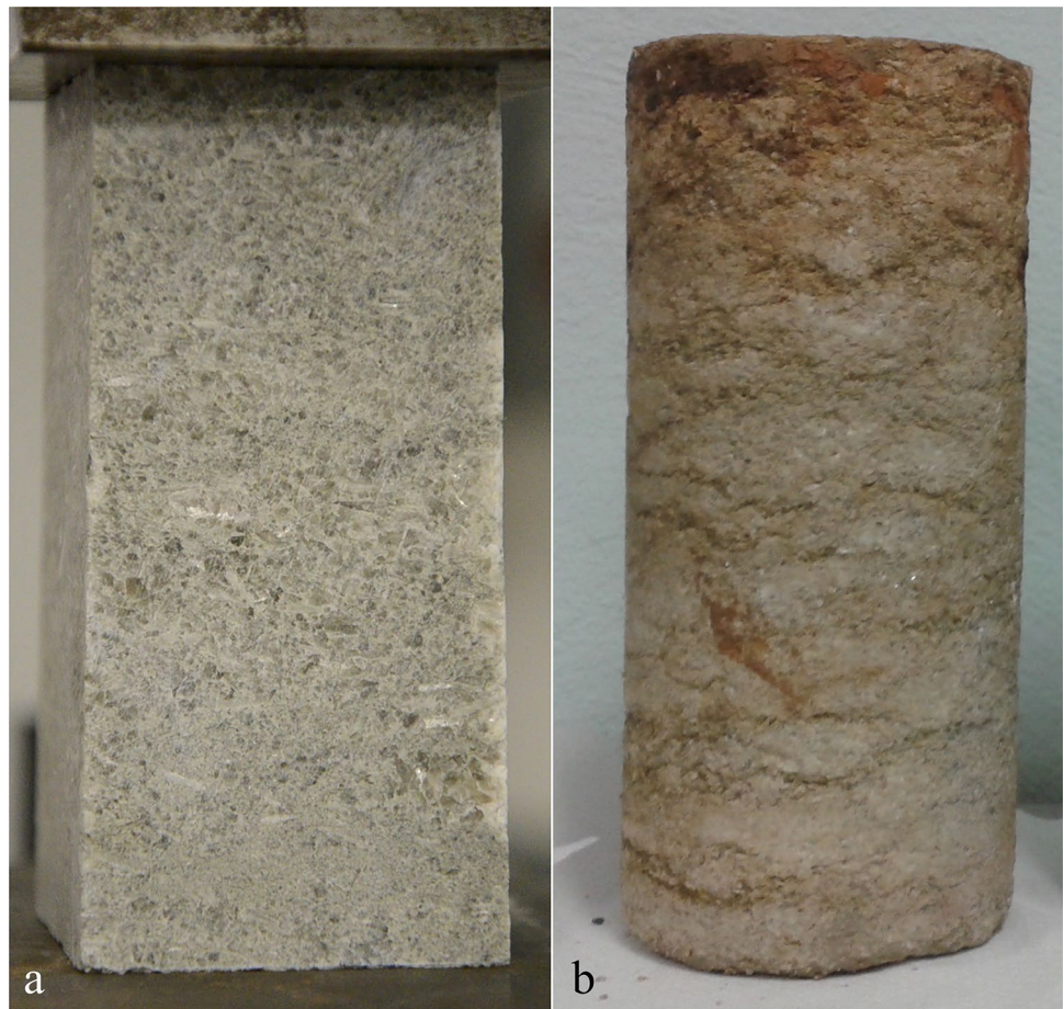
Fig. 2 Samples of branching selenite gypsum, underlining the mesoscopic heterogeneity of the material
