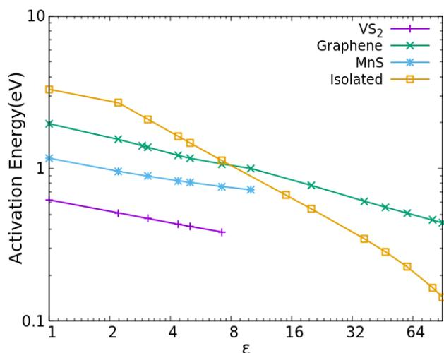
**Figure 7:** Activation energy for breaking the Li-S bond of the  $\text{Li}_2\text{S}$  molecule in the absence of a surface and on graphene,  $\text{VS}_2$  and  $\text{MnS}$  surfaces, with different values of dielectric constant.
