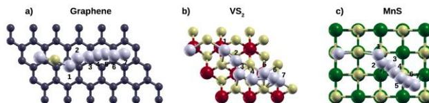
**Figure 3:** Trajectories of the Li atom being separated from the  $\text{Li}_2\text{S}$  molecule on a) graphene, b)  $\text{VS}_2$  and c)  $\text{MnS}$  surfaces. The numbers on the graphs indicate the configuration of the lithium atom corresponding to the image in the reaction coordinate of the NEB path. C atoms are black, S atoms are yellow, V atoms are red, Mn atoms are green, and Li atoms are light blue.
