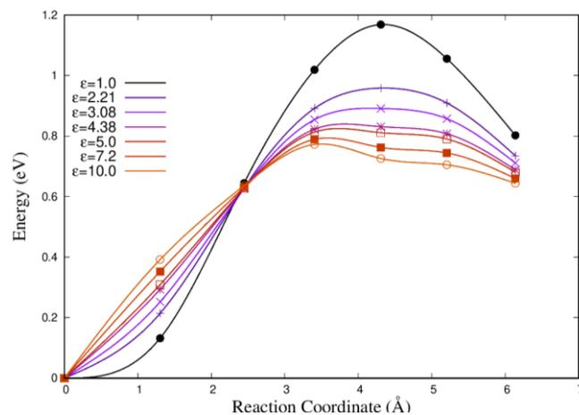
**Figure 6:** Decomposition energy barrier as a function of the reaction coordinate for a  $\text{Li}_2\text{S}$  molecule adsorbed on  $\text{MnS}$  in contact with different solvents, represented by their dielectric constant.
