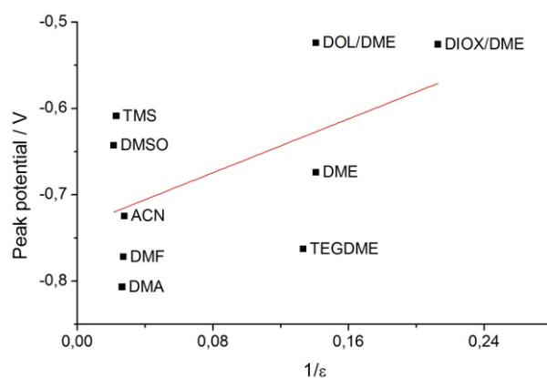
**Figure 8.** Peak potential for the most positive voltammetric oxidation peak observed on a glassy carbon electrode under an argon atmosphere at room temperature in various organic solvents with dissolved S<sub>8</sub>, as a function of the inverse dielectric constant. Data were taken from reference [31]
