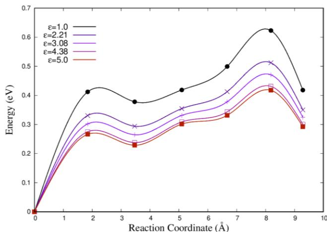
**Figure 5:** Decomposition energy profile as a function of the reaction coordinate for a  $\text{Li}_2\text{S}$  molecule adsorbed on  $\text{VS}_2$  in contact with different solvents, characterized by their dielectric constant  $\epsilon$ .
