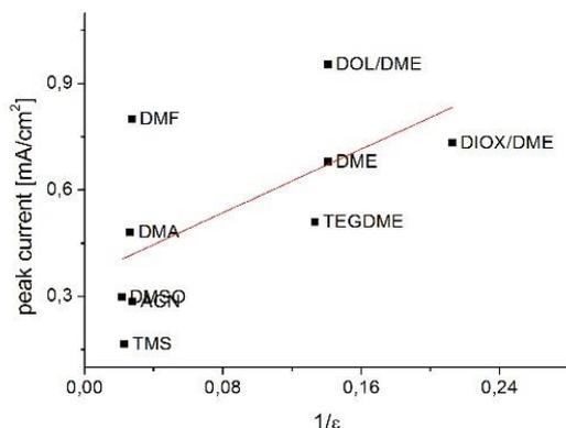
**Figure 9:** Peak current density for the most positive voltammetric oxidation peak, observed on a glassy carbon electrode under an argon atmosphere at room temperature in various organic solvents with dissolved  $S_8$ , as a function of the inverse dielectric constant. Data were taken from reference [31]
