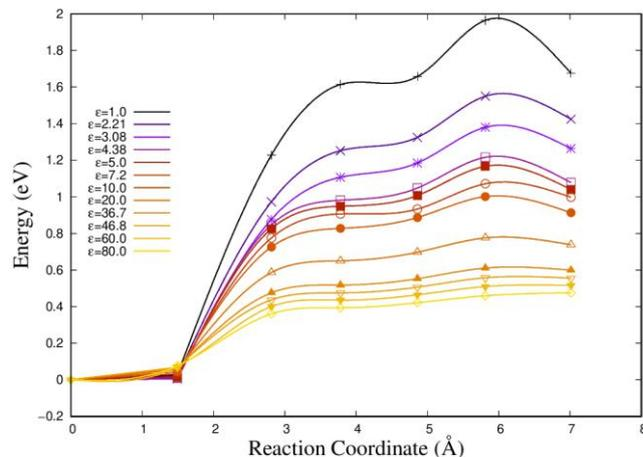
**Figure 4:** Decomposition energy profile as a function of the reaction coordinate for a  $\text{Li}_2\text{S}$  molecule adsorbed on graphene in contact with different solvents, characterized by their dielectric constant,  $\epsilon$ .
