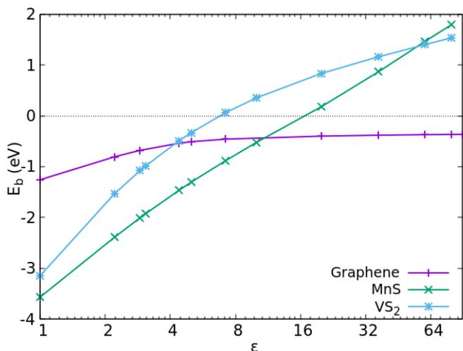
**Figure 1:** Binding energy of a  $\text{Li}_2\text{S}$  molecule on different surfaces immersed in a dielectric as a function of the logarithm of the dielectric constant.
