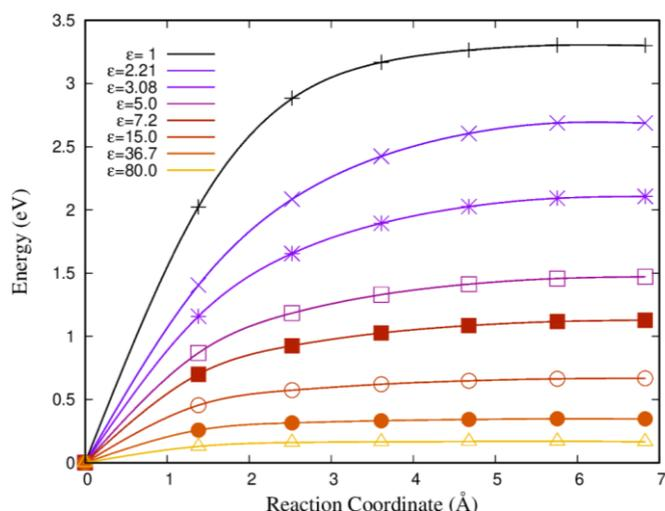
**Figure 2.** Energy profiles for the decomposition reaction of a single isolated (in the absence of a surface support)  $\text{Li}_2\text{S}$  molecule as a function of the reaction coordinate for different values of  $\epsilon$  in the range 1 - 80.
