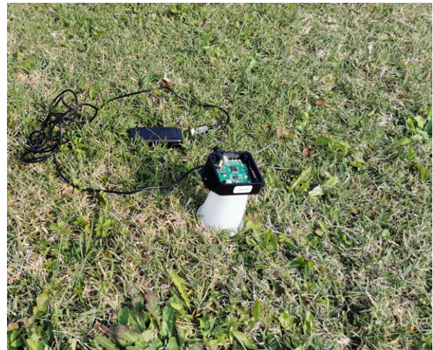
Figure 2. Example of Pozyx UWB anchor.
