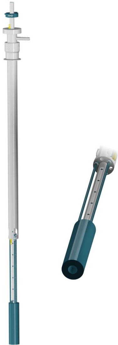
Figure 1. A computer rendering of the cryomagnetic probe assembly: (left) side view; (right) front view, showing the magnet bore.
