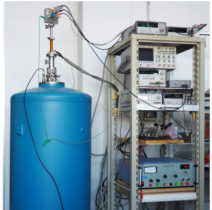
Figure 7. Overall view of the measurement setup for DC characterization. On the left, the liquid helium dewar, with the coaxial probe inserted. On the right, the rack of electronic instrumentation.
