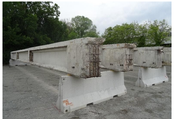
Figure 16. PC beams testing site arrangement.
