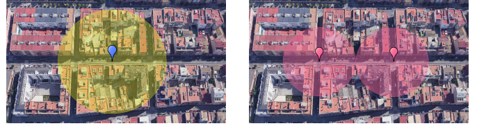
Fig. 4. Map of the geographical area served by the EVS service, featuring two intersections and including an IEEE802.11p RSU: one EVS instance and corresponding covered intersections highlighted in yellow (left), two EVS instances and corresponding covered intersections highlighted in pink (right)
