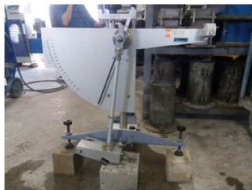
Figure 7. Investigation of different RCCP micro/macro-textures by British pendulum test setup.
