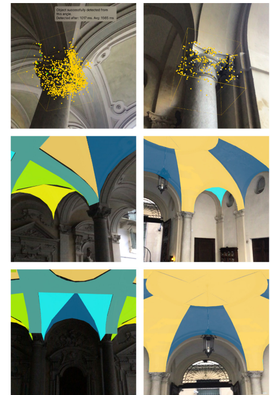
Fig. 6 - Scanning of target object features and superimposition of 3D models in the palaces d'Arcour and Coardi di Carpenetto. Illustration by V. Palma.
