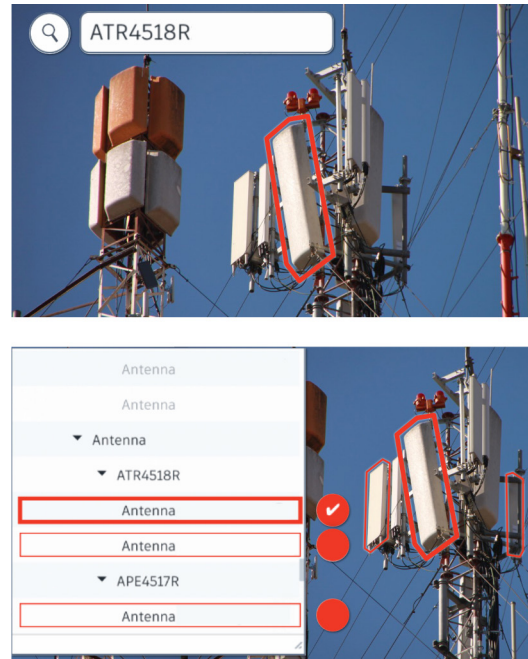
Fig. 10 – Example of planned model selection methods: searching an element by identification code (top), selection from model browser (bottom). Illustration by V. Palma.
