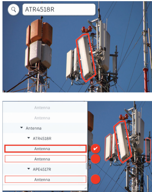
Fig. 10 – Example of planned model selection methods: searching an element by identification code (top), selection from model browser (bottom). Illustration by V. Palma.
