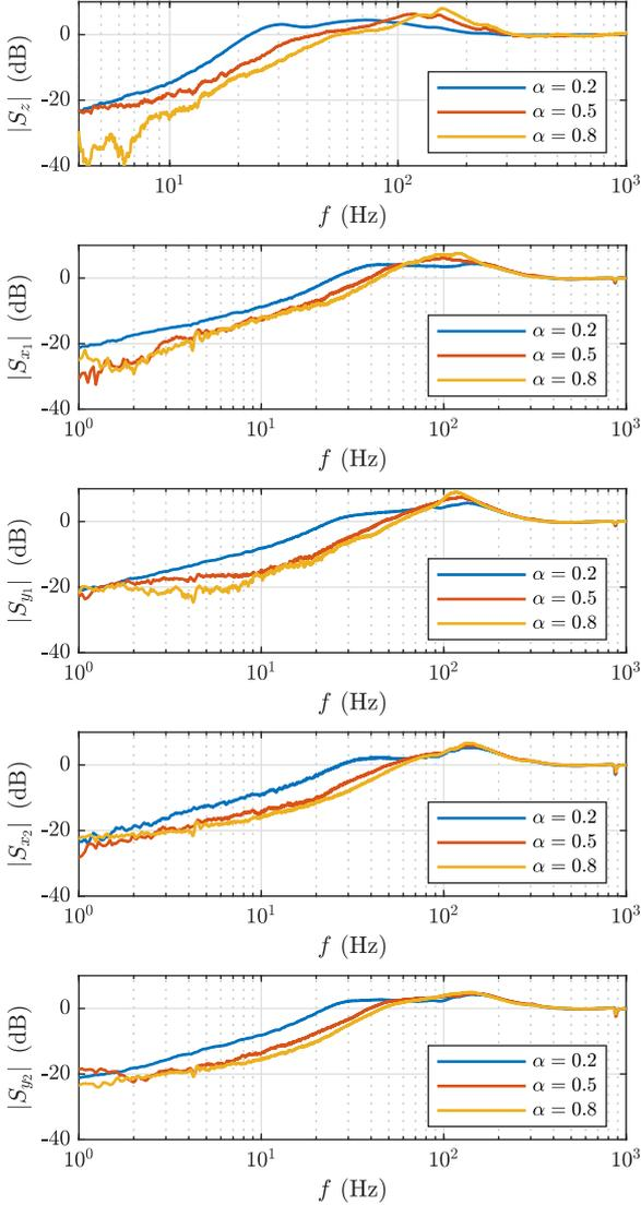
Figure 8: Output sensitivities on  $z$ ,  $x_1$ ,  $y_1$ ,  $x_2$  and  $y_2$  for different grades of controller aggressiveness  $\alpha_{z,x_1,y_1,x_2,y_2} \equiv \alpha$ . Each test is performed independently on each measurement channel by injecting a sweep noise with a frequency that varies from 0.1 Hz to 1 kHz and amplitude  $10 \mu\text{m}$ .
