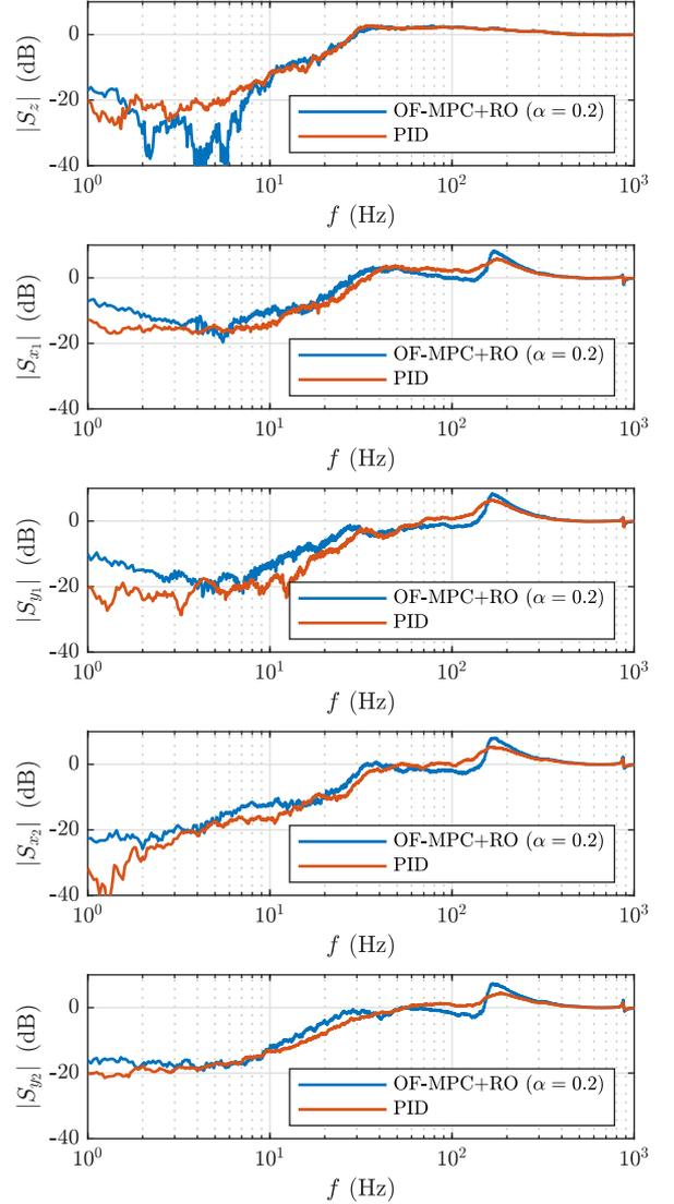
Figure 10: Output sensitivities on  $z$ ,  $x_1$ ,  $y_1$ ,  $x_2$  and  $y_2$  from a comparison of the OF-MPC + reduced observer (RO) with decentralized PID controllers. Each test is performed independently on each measurement channel by injecting a swept sine noise with a frequency that varies from 0.1 Hz to 1 kHz and an amplitude 10  $\mu$ m.
