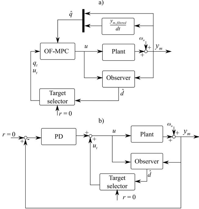
Figure 9: a) OF-MPC with a reduced observer (RO) i.e., only the disturbance estimates  $\hat{d}$  are obtained from the observer.  $\hat{q}$  is obtained directly from the measurements. b) Control scheme with PID controllers. The integral action is identical to that of the OF-MPC.
