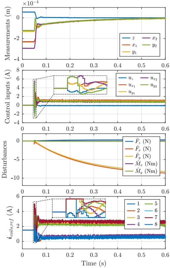
Figure 7: Transient response when the plant lifts-up. Control aggressiveness is set to  $\alpha_j = 0.2$ . The zoomed area evidences the coil current saturation together with the corresponding control inputs.
