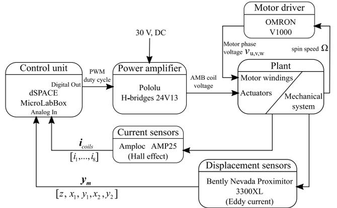
Figure 6: Block diagram of the test bench.
