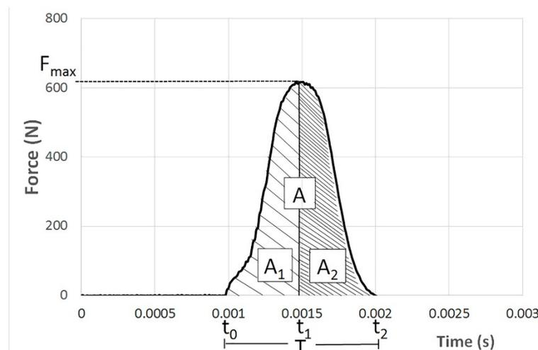
**Figure 6.** Example of force–time diagram in impact test.
