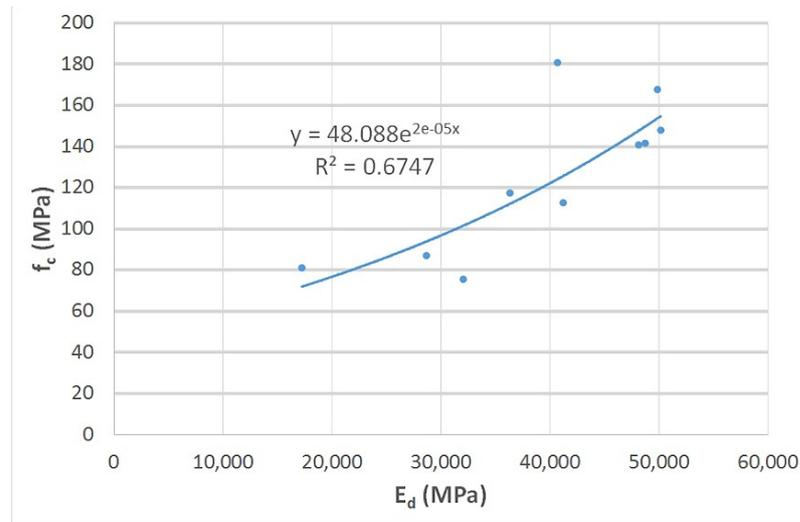
**Figure 12.** Exponential correlation between cylindric compression strength and dynamic elastic modulus.
