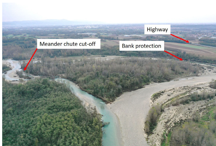
FIGURE 5 A meander chute cut-off on the Orco River near San Benigno Canavese village, Italy (Source: Paolo Maschio, Politecnico di Torino)
