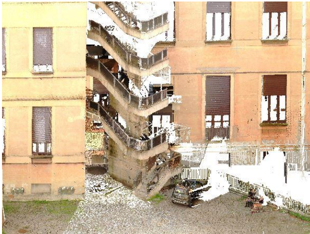
Figure 5. TLS scans of the test area composing the dataset (c).
