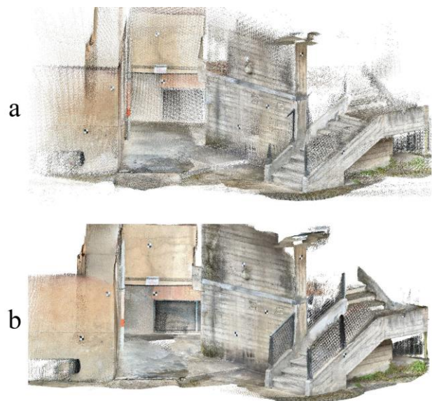
Figure 3. Point clouds of the dataset (a) composed by a single iPad Pro scan with lowest resolution, and dataset (b) composed by 7 overlapping point clouds with highest resolution in SiteScape app.
