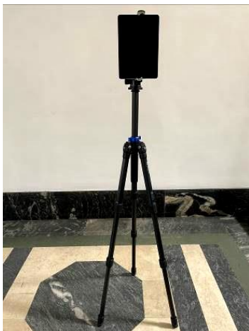
Figure 1. Static configuration of the iPad mounted on a tripod to acquire the white vertical wall.
