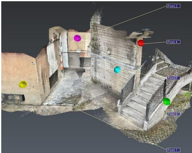
Figure 11. GCPs collimated in the point cloud (A) to evaluate the 3D accuracy on measured points.
