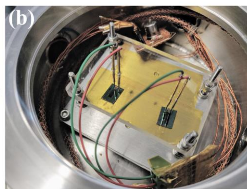
Figure 2: (a) Scheme of the experimental sensing setup used to perform gas sensing measurements (b) Interior of the gas detection chamber.
