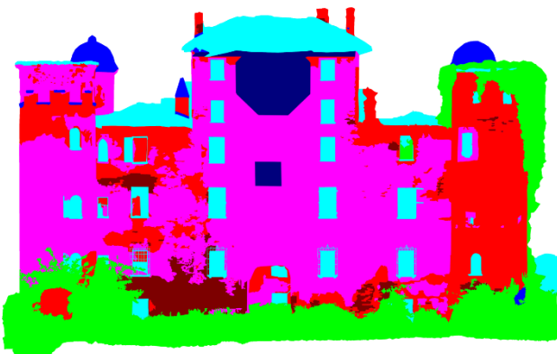
Figure 12. Orthophoto manually labelled by an operator, serving as ground truth to evaluate the results.
