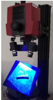
Figure 5. Inspection of a cantilever using the Atos Compact Scan 2M.
