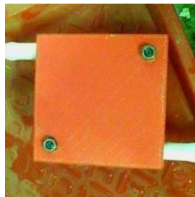
Figure 2. 3D printed heat exchanger with ABS casing and PA12 duct.
