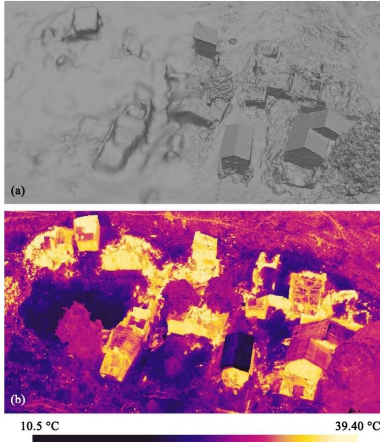
**Fig. 4.** (a) Level of detail differences between the mesh obtained from thermal dataset only (on the left) and optical dataset (on the right). (b) 3D mesh obtained from optical dataset texturized with co-registered thermal images.
