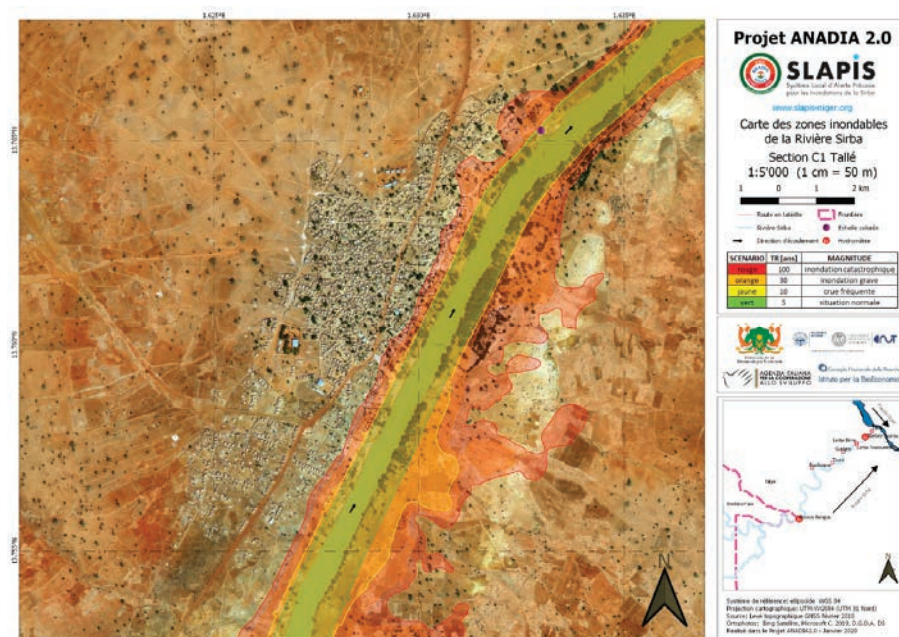
Figure 4. Atlas of flood-prone areas of the Sirba river. Tallé village (Gotheye municipality, Niger). This image reproduces the Table C1 of the Atlas which is in the official language of Niger (French). The Atlas is annexed as a Supplementary Material.
