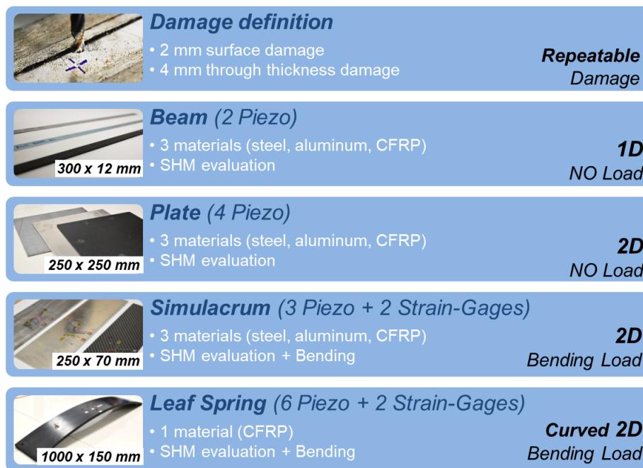
Figure 0.1 – Damage types and geometries studied in the Thesis
