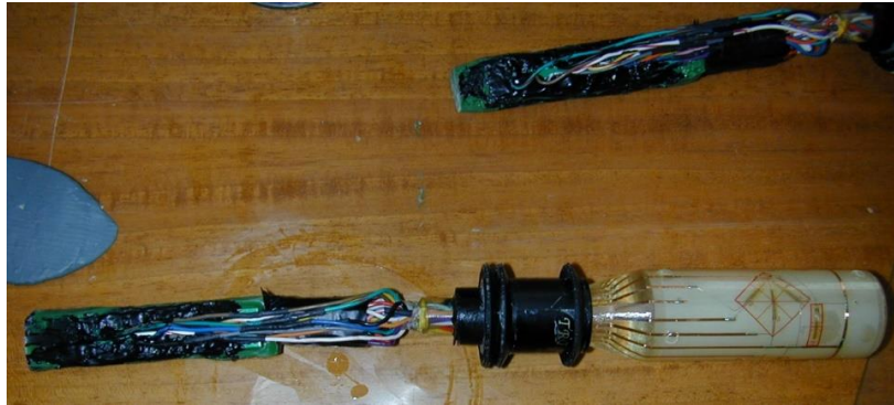
Figure 2. Picture showing the connection between the micro12 measuring device and a generic HI cell. The rechargeable batteries that energize the whole system are also visible.
