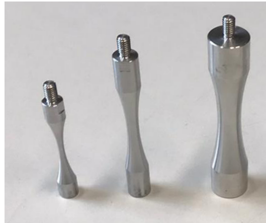
Figure 2. The three different investigated hourglass-specimens.
