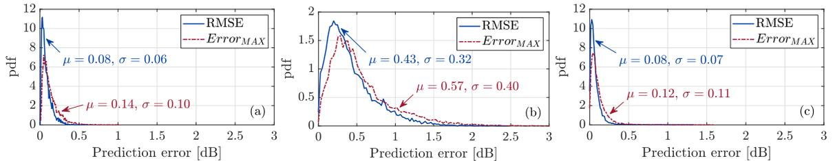
Fig. 2: Probability density functions of  $RMSE$  and  $Error_{MAX}$  for: (a) LU-NN validated over full load cases only, (b) LU-NN validated over the entire data-set, and (c) LA-NN validated over the entire data-set.
