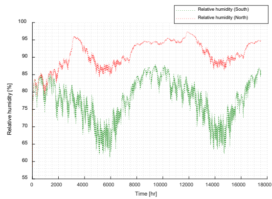
Fig. 6 – Relative humidity trend on the cellulose - external perforated brick interface. Results from 2-year dynamic simulation
