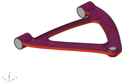
Figure 30. Plies after shuffle optimization
