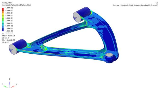
Figure 32. Contour plot of composite bond failure: braking load case (shuffle optimization)
