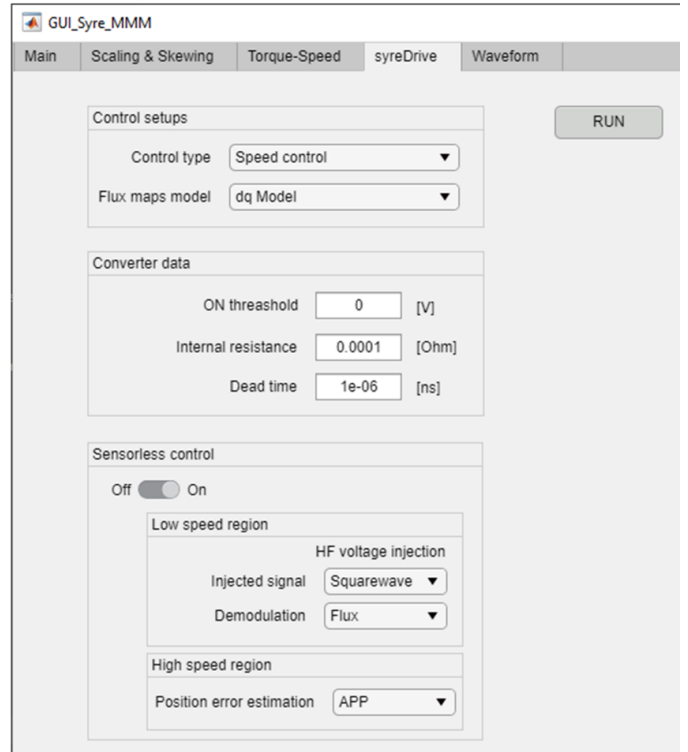
Fig. 2. Graphical user interface of syreDrive within the SyR-e magnetic model manipulation framework.
