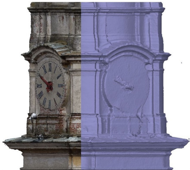
Figure 8: Portion of the 3D model derived from the UAVs dataset processing: point cloud (left with RGB value) and mesh model (right in violet).
