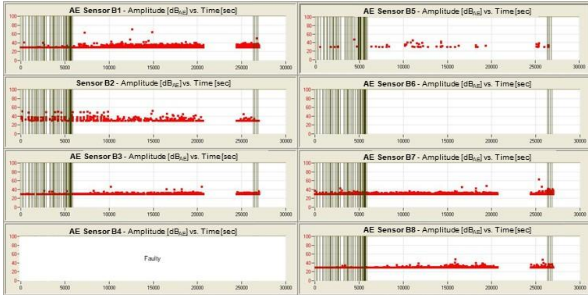
Figure 15: AE recording during 8-h monitoring under normal traffic: amplitude vs. time (screen shot of the acquisition software) [61].
