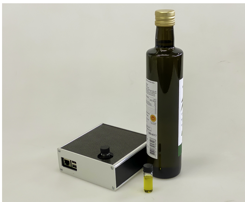
Figure 2. Photo of the minimalist fluorescence sensor with olive oil samples in the glass vials and a bottle of olive oil.
