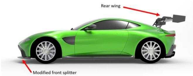
Figure 4 - New reference vehicle aerodynamic interventions
