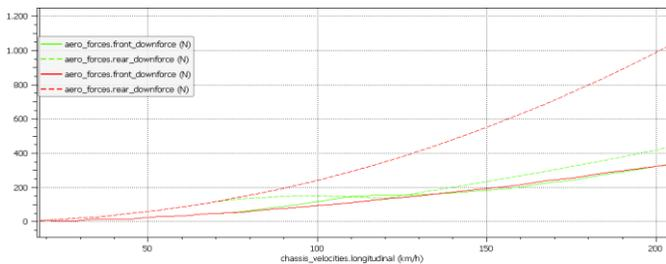
Figure 9 – Downforces vs. speed, Passive (red) and DRS operation (green), straight acceleration
