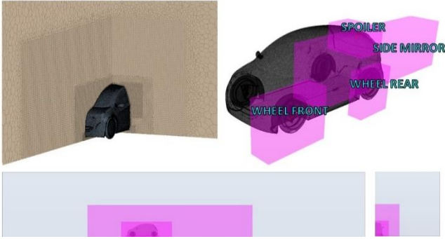
Figure 2 - Mesh volume refinements
