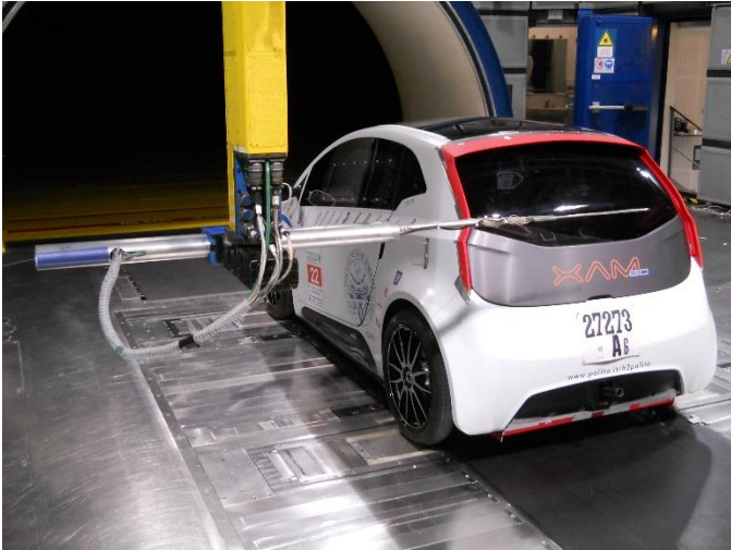
Figure 5 - Pressure field measurement with 14-holes probe
