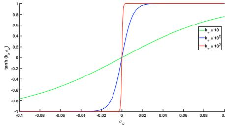
Fig. 1. Effect of  $k_\sigma$  on the  $\tanh$  function
