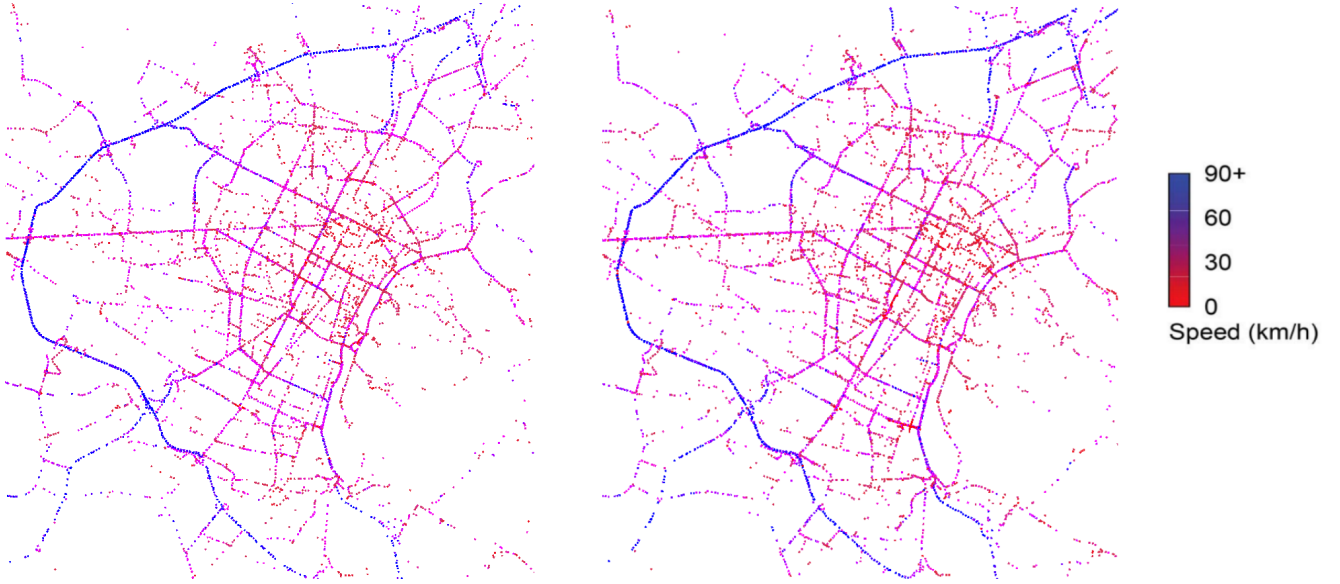
Fig. 3. Snapshots from the final TuST dataset. Red vehicles are slow or stopped, blue ones are moving fast. Morning peak of 8:00am (left) and afternoon peak of 17:00pm (right).
