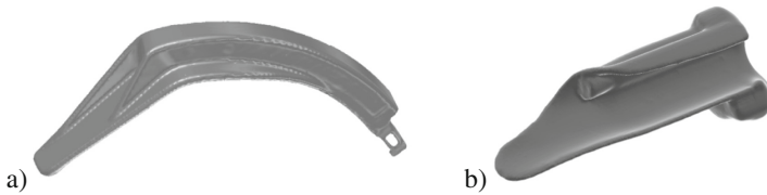
Fig. 2. Scanned Blades: a) adult blade; b) pediatric blade.
