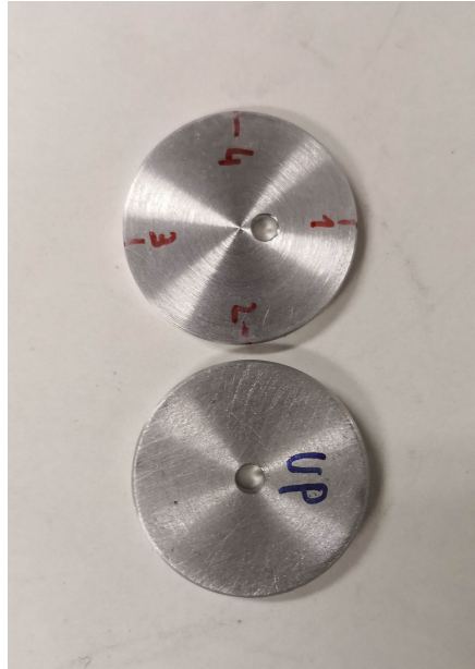
FIGURE 4.11: The two collimators used to analyse small sample areas.
