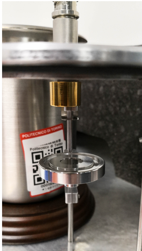
FIGURE 4.9: The internal part of the vacuum chamber, with the holder for the source and the sample, and the silicon detector.
