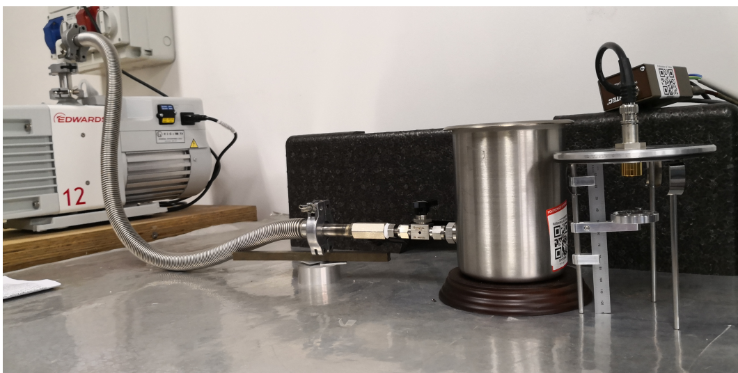
FIGURE 4.10: The internal and external parts of the vacuum chamber, disassembled, and the connection to the vacuum pump.
