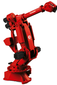
Fig. 1: A robotic manipulator (Comau SMART NJ 650).
