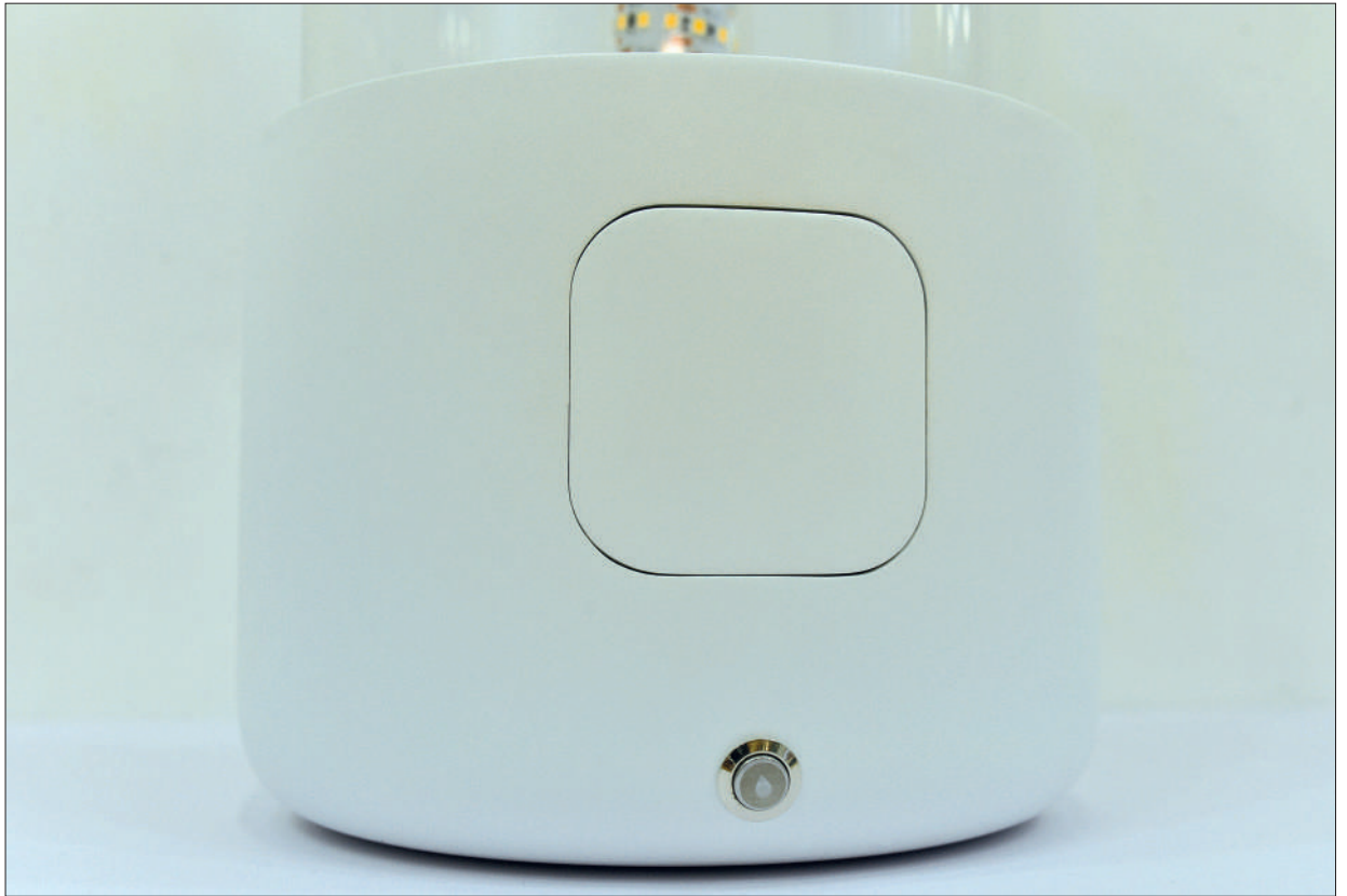
Detail of the front of the device: closed drawer and Spirulina harvesting button.
