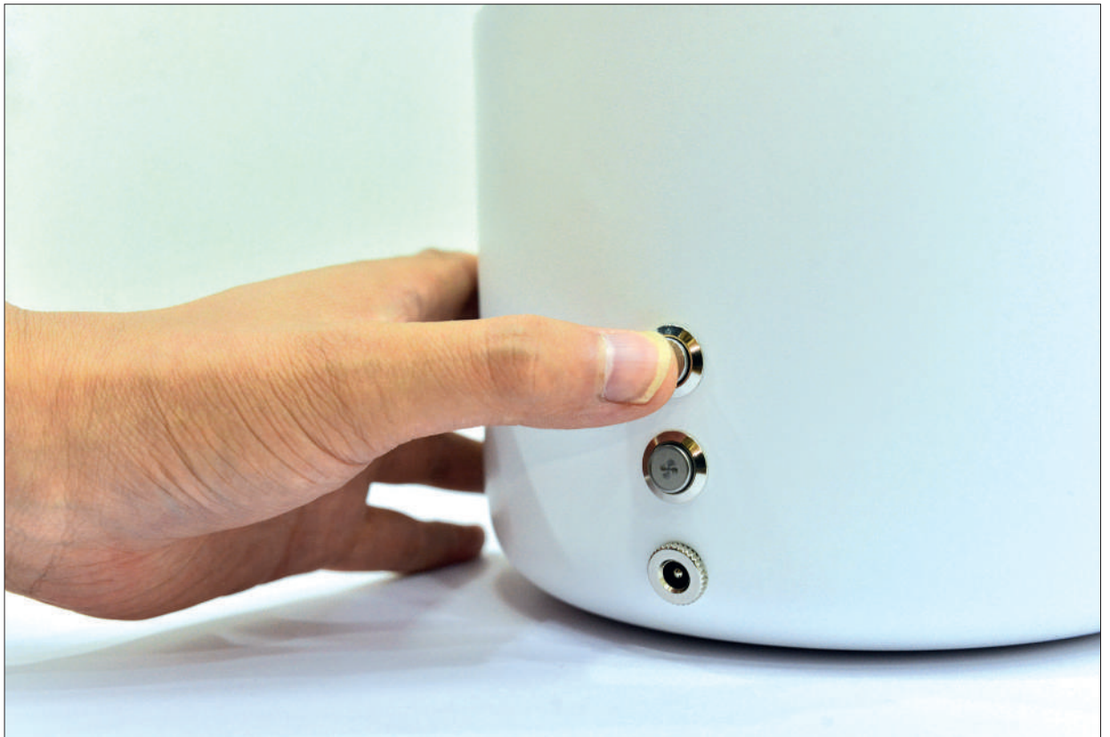
Buttons on the back of the device and power plug socket connector. Icons are laser-engraved on the buttons.
