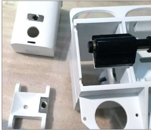
Details of the extractable drawer and the magnetic buckle mechanism.
