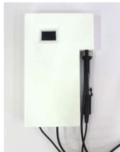
Figure 8.19. The 3D-printed shell that includes temperature and pH sensor, to be used for monitoring the parameters of the culture.
