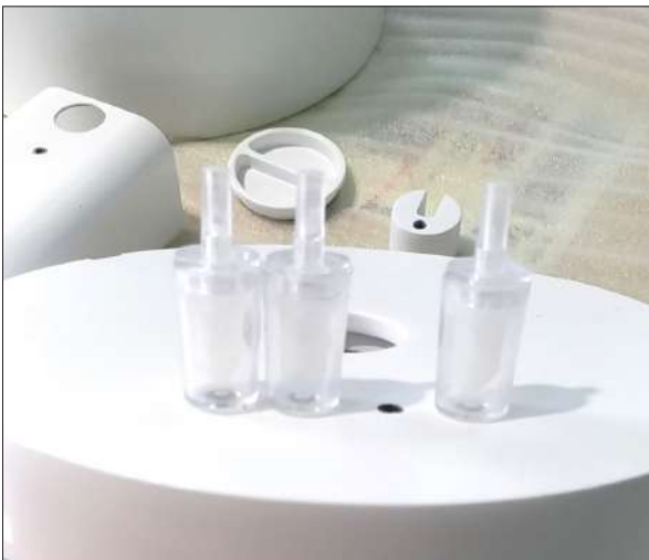
Water check valves.
