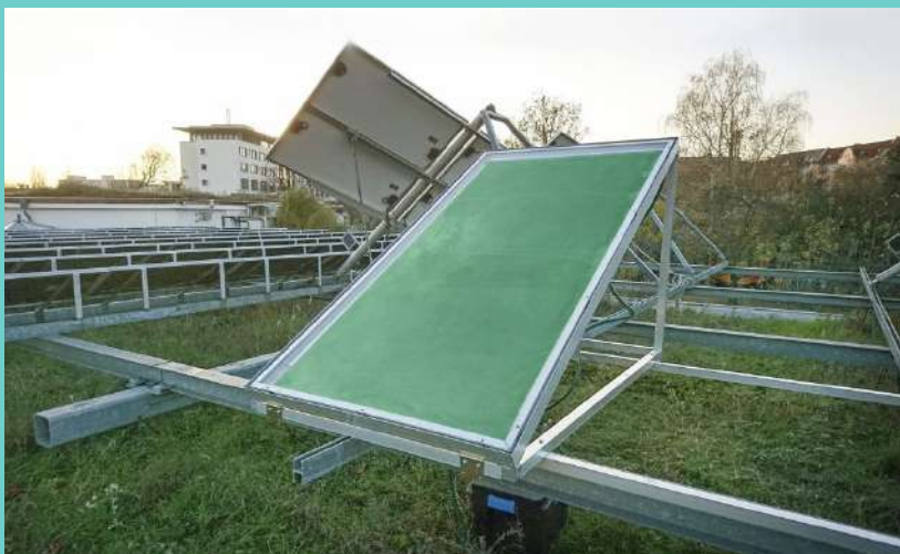
Figure 7.71. A flat panel PBR for the production of solar biogas is tested in Solaga facilities.
