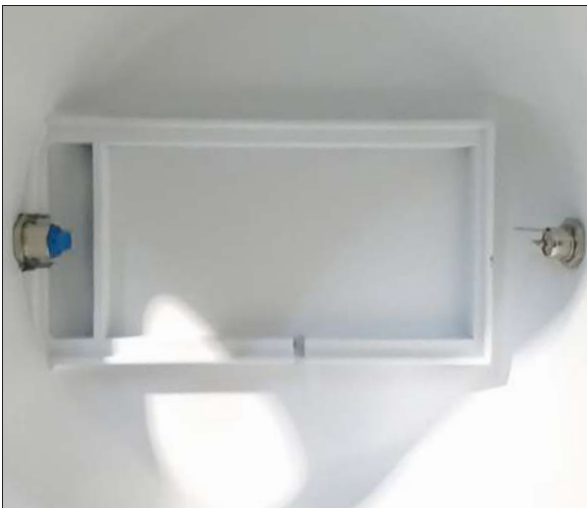
The connections on the inner part of the lower main body, with the front button and the power connector.
