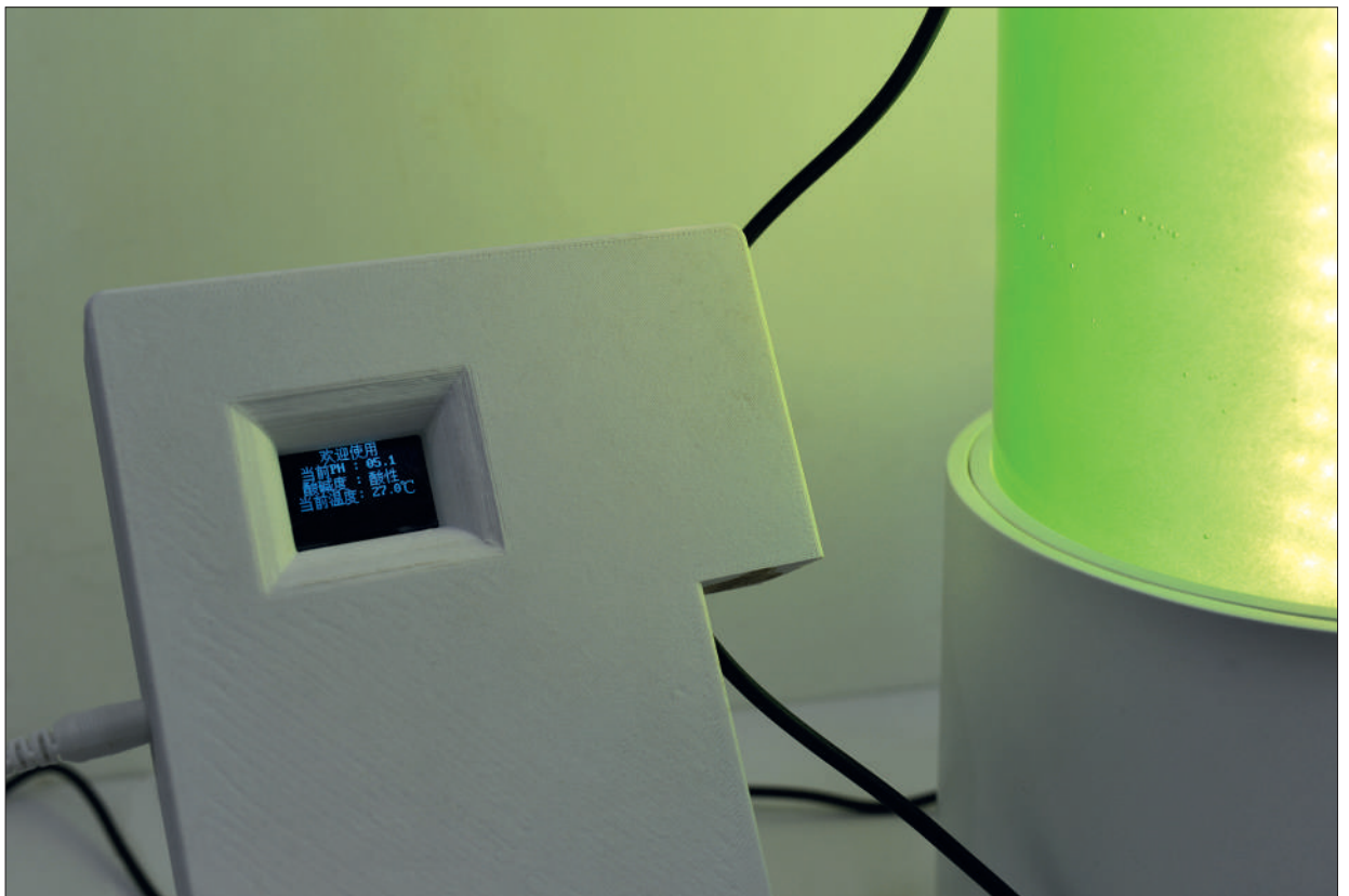
External pH and temperature sensors, measuring culture parameters.
