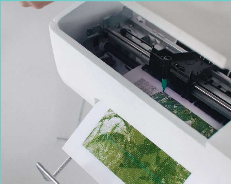
Figure 7.14. CMYKA is an algae dying system using an ink-jet printer. Adapted from Edinburgh College of Art - Product Design website, 2016, retrieved from https://sites.eca.ed.ac.uk/designnarratives/algae-the-shape-of-things-to-come/ Copyright 2016 by Leon Brown.
