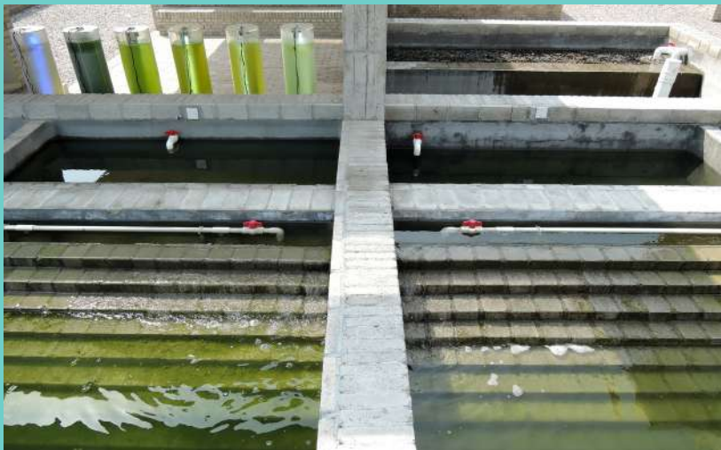
Figure 7.56 (Left). Microalgae are harvested to produce fish feed and to improve the purification of the water.
