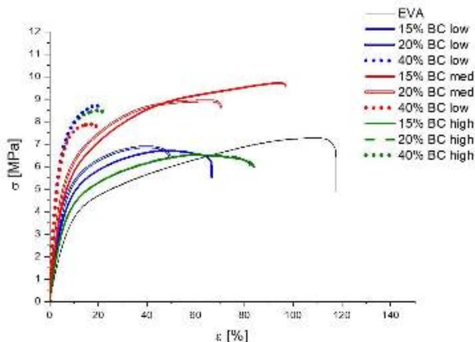
Figure 7. Stress–strain curves for EVA and EVA/BC compounds.
