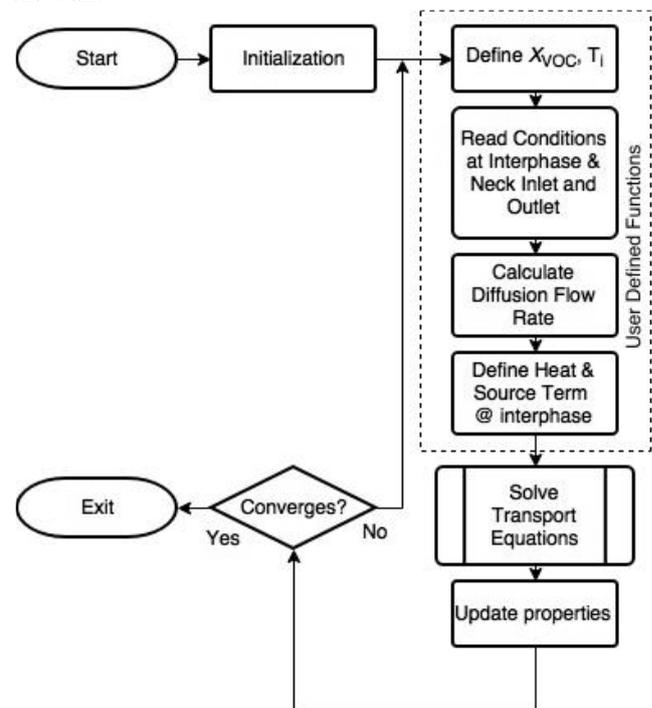
Fig. 3. Simplified Flowchart for ANSYS Fluent Calculation
