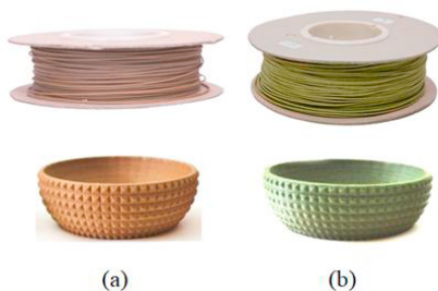
Fig. 2. Thermoplastic bio-composite filaments: (a) HEMP; (b) WEED.
