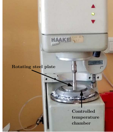
Figure 4: Rheometer test set-up
