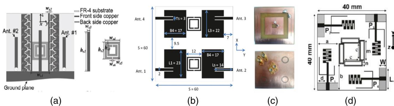
**Figure 1.** (a) Square SRR at the back (J. Y. Lee et al., 2015) (b) Pair of SRRs between the antenna (A. Kumar, Ansari, Kanaujia, & Kishor, 2018) (c) CSRRs loaded in its ground plane (Ramachandran et al., 2016) (d) A ring of four SRRs (Ramachandran et al., 2017). CSRR, complementary-split-ring-resonator; SRR, split-ring-resonator.
