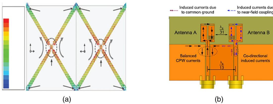
**Figure 19.** (a) X-shaped etched arms (H. Wang et al., 2015) (b) MTM-inspired MIMO antenna (Jiang, Zhu & Eleftheriades, 2010). MIMO, multiple-input-multiple-output; MTM, Metamaterials.
