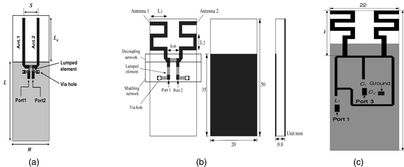
**Figure 9.** (a) Two TLs with reactive shunt component (Lin et al., 2012) (b) decoupling network along with a lumped element (Cui et al., 2011) (c) hybrid ring of arbitrary power division (Gong et al., 2011).
