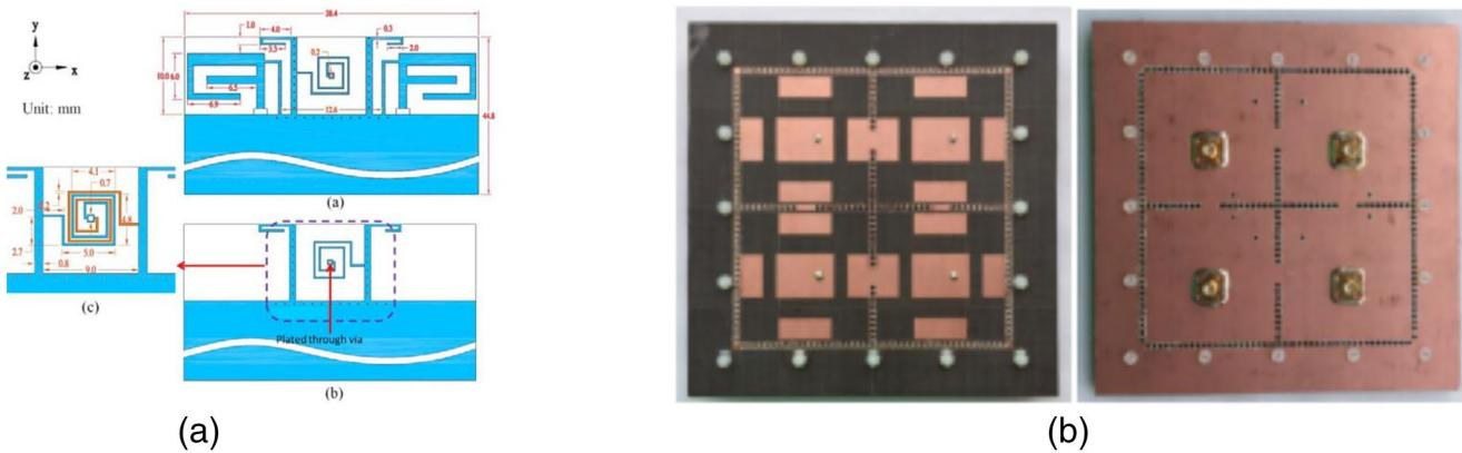
**Figure 6.** (a) Compact planar spiral line (PSL) structure (Xun et al., 2017) (b) metallized via walls and short-circuited stepped-impedance structures (K. Da Xu et al., 2018).
