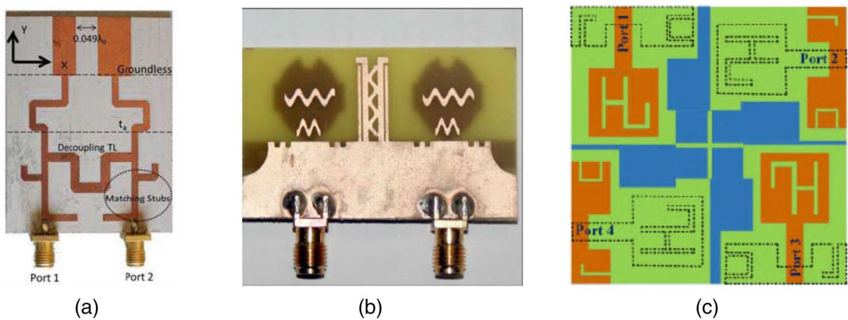
**Figure 8.** (a) A novel and general decoupling network (Moharram & Kishk, 2013) (b) sinusoidal decoupling structure (Bilal et al., 2014) (c) a novel decoupling structure along with DGS, slots & slits (Z. Tang et al., 2019). DGS, defected ground structures.
