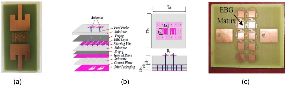
**Figure 5.** (a) A novel uni-conductor EBG placed between patch antenna (Mohamed et al., 2019) (b) a novel EBG ground (Shen et al., 2019) (c) 2 × 5 EBG structure (Islam & Alam, 2013). EBG, electromagnetic band gap.
