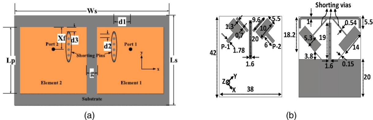
**Figure 17.** (a) Six pairs of shorting vias (Abdullah et al., 2019) (b) metallic strip along with shorting vias (Sipal et al., 2019).
