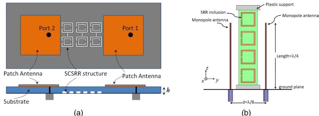
**Figure 2.** (a) Slotted CSRRs (Bait-Suwailam, Siddiqui, et al., 2010) (b) Single negative (MNG) MTMs (Bait-Suwailam, Boybay, et al., 2010). CSRR, complementary-split-ring-resonator; MTMs, Metamaterials.
