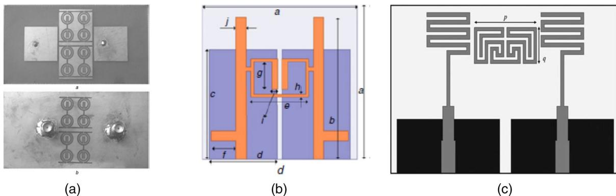
**Figure 3.** (a) Slot combine CSRR on surface and ground (Qamar et al., 2014) (b)  $\mu$  negative MTM filter (Thummaluru & Chaudhary, 2017) (c) Labyrinth SRR (Torabi et al., 2016). CSRR, complementary-split-ring-resonator; MTM, Metamaterials.
