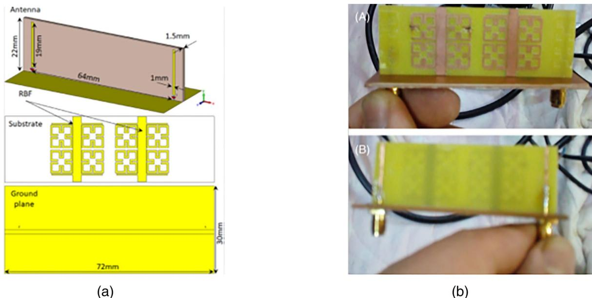
**Figure 14.** (a) Designed two RBF (b) Fabricated monopole MIMO antenna with the two RBF (Ahmed & Elwi, 2019). MIMO, multiple-input-multiple-output; RBF, reject band filter.
