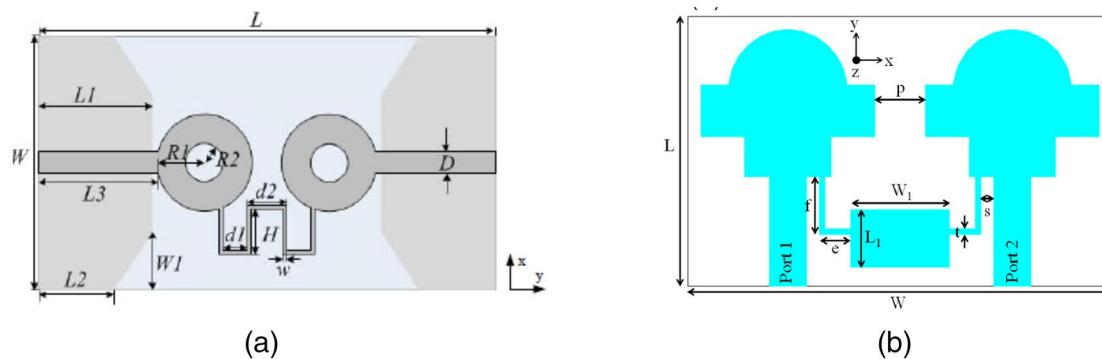
**Figure 11.** (a) Meandered-shaped metallic NL (Y. Yu et al., 2016) (b) NL comprises of two metallic strips and a rectangular patch (Tiwari, Singh, & Kanaujia, 2019; Tiwari, Singh, & Kanaujia, 2019). NL, neutralization line.
