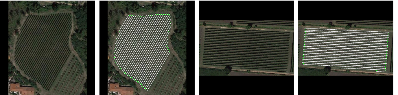
Fig. 3: Two examples of real-world images taken from Google Maps satellite database and manually annotated. Green points are the ground truth waypoints computed with the method presented in Fig. 1.
